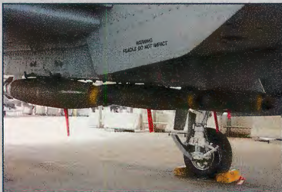
(top) Quite a snout on an A-10 "Warthog." A 30mm eight-barrelled cannon can make swiss cheese of enemy armored vehicles with its uranium-depleted armor-piercing ammunition. (above) Four 500-pound bombs under belly of Thunderbolt II at a forward air base in the Persian Gulf. These aircraft, and others, will provide close-air support for U.S. Army units inside Iraq.
